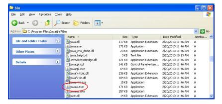
Right click on the javaw.exe shortcut and select Properties. On the Shortcut TAB, edit the target field to include the information needed to launch SwitchCenter. For Example:
