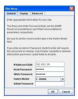
After you enter the IP address, SNMP read and write community names (passwords), select the appropriate Switch Model for your switching system, enter an optional Admin Password, then click OK.
